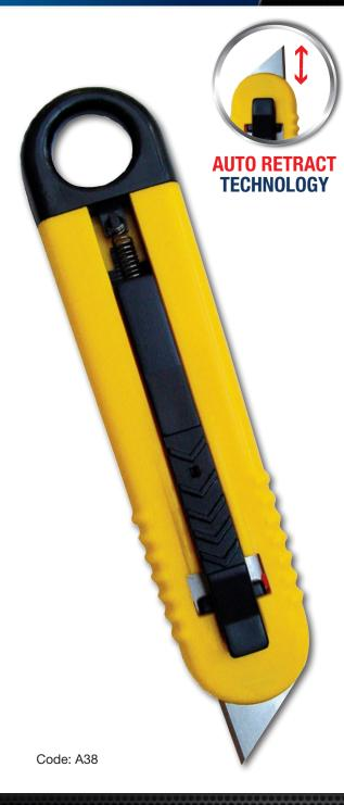
A38LH safety knife is a budget cutter featuring a springloaded mechanism, which allows the heavy-duty utility blade to automatically retract into the knife. A38LH has universal application and meets the industry requirements for the use of safety knives to reduce the risk of workplace accidents.
